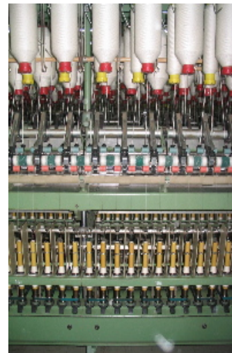
Right: Ring spinning frame producing cotton yarn
